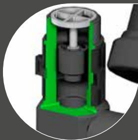
Automatic Switching Flow Switch – automatically starts the pump when flow exceeds 1 litre/min
