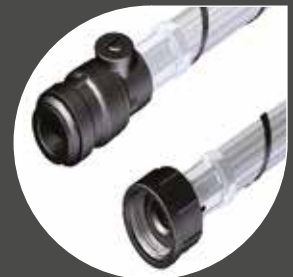
Flexible Hoses 200 mm anti-vibration flexible hoses with integral isolating valves G 3/4 threaded connections to pump 15 mm push fit to pipe work
