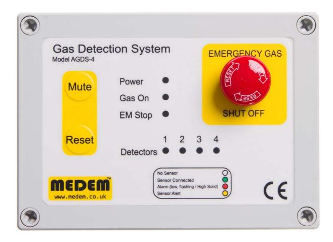
The AGDS-4, Gas detection system has been designed for use in boiler houses and plant rooms. Up to 4 low voltage sensors for the detection of natural gas, LPG or carbon monoxide can be connected to the panel. In the event of a high alarm from one of the sensors the system will isolate the gas supply by closing a connected electric control valve. Emergency stop buttons can be fitted and a fire alarm can close the gas valve when connected to the panel.
