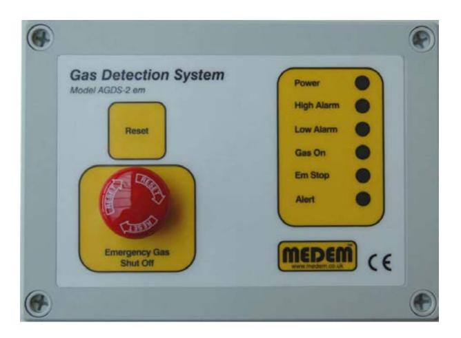
The AGDS-2em, Gas detection system has been designed for use in boiler houses and plant rooms. Up to 2 low voltage sensors for the detection of natural gas, LPG or carbon monoxide can be connected to the panel. In the event of a high alarm from one of the sensors the system will isolate the gas supply by closing a connected electric control valve. Emergency stop buttons can be fitted and a fire alarm can close the gas valve when connected to the panel.
